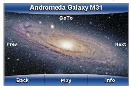
Push the soft key labeled PLAY for audio descriptions, video, and images of the object or INFO for on-screen text data about the object. To exit a tour: Press the key labeled END TOUR. If the END TOUR option is not displayed, keep pressing the BACK key until END TOUR is displayed.
